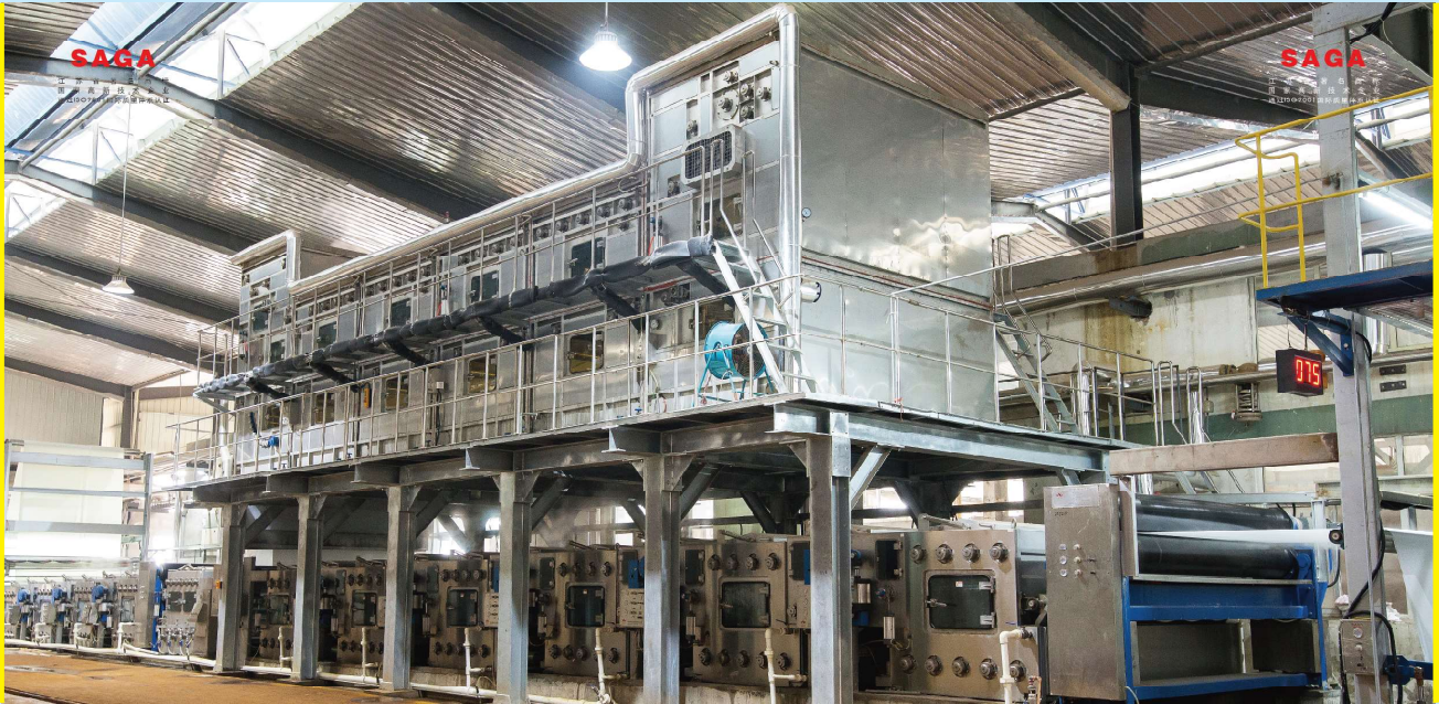
DESIZING SCOURING AND BLEACHING RANGE
